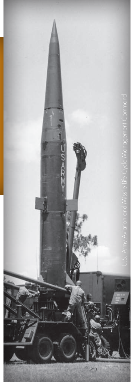
Right and page 9: A Pershing 1A missile sits atop its wheeled erector-launcher at the Orlando Division facilities of the Martin Marietta Corporation in Florida, April 1969.
